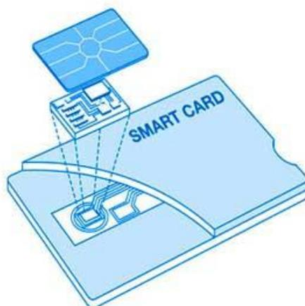
The most important challenger to mention is the quickly rising Smart Card technology<sup>9</sup>. Smart cards look a lot like magnetic stripe cards, but instead of storing data on a ferromagnetic stripe, they use embedded memory or microcontrollers to store or even process data within the card itself. Smart cards come in many flavors; some have external pin contacts which connect the
